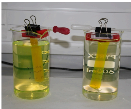
Figure 14: First rinse water from cellulose dialysis tubing. The more yellow (left) is funori.
