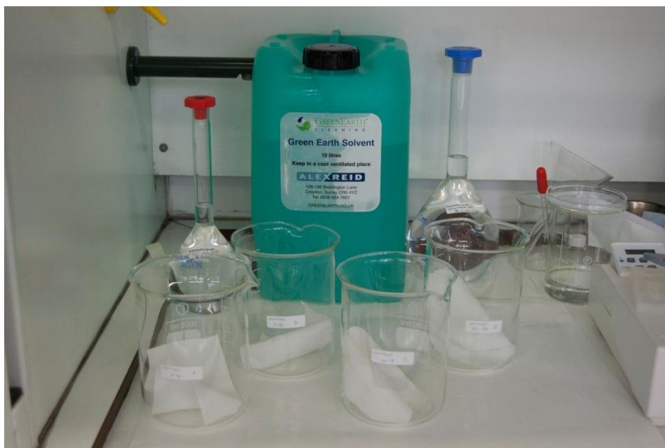
FIGURE 2.3: MATERIALS ASSEMBLED IN FUME CUPBOARD IN PREPARATION FOR D5 IMMERSION TREATMENT.
