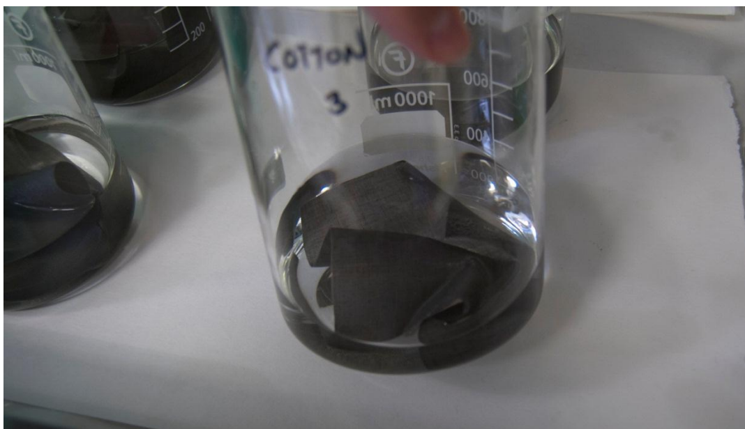
FIGURE 2.9: IMMERSION TREATMENT OF SOILED COTTON SAMPLE
