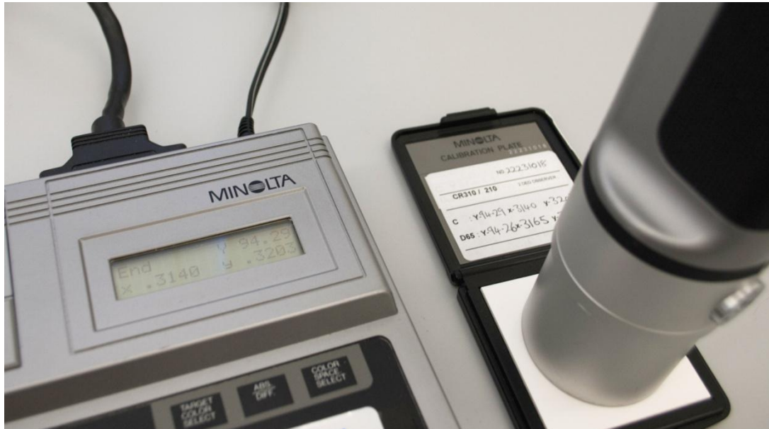
Figure 5.5 Calibration of the chroma meter using the white calibration tile.
