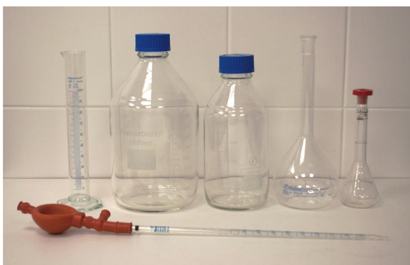
Figure D.1 Glassware used in the preparation and storage of wash solutions and pH buffers, and to measure out each wash bath.
