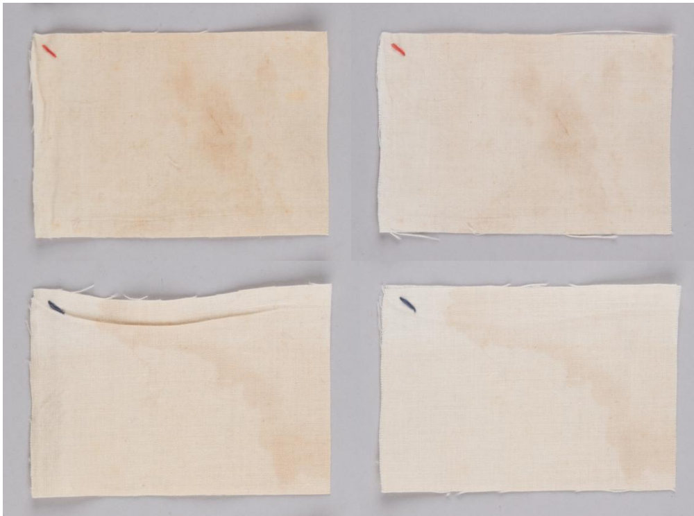
Figure 6.5 Before (left) and after (right) wet cleaning of samples HS2 (top) and W2 (bottom).
