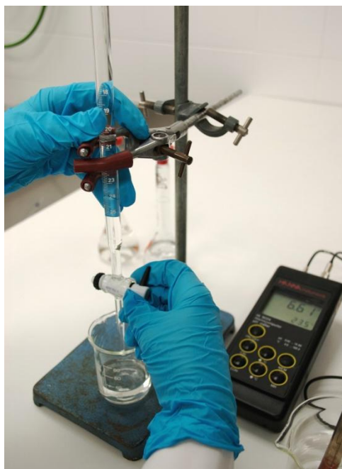
Figure 5.8 Titration to adjust pH of sodium hydroxide with citric acid buffer.
