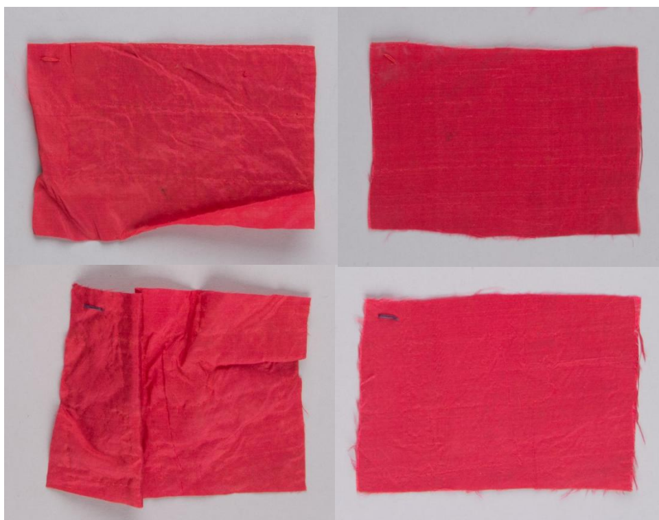
Figure 6.10 Before (left) and after (right) wet cleaning of samples DS2 (top) and W3 (bottom).
