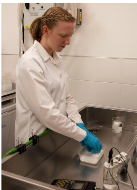
Figure 5.9 Wet cleaning cotton sample with Hostapon T® wash solution.
