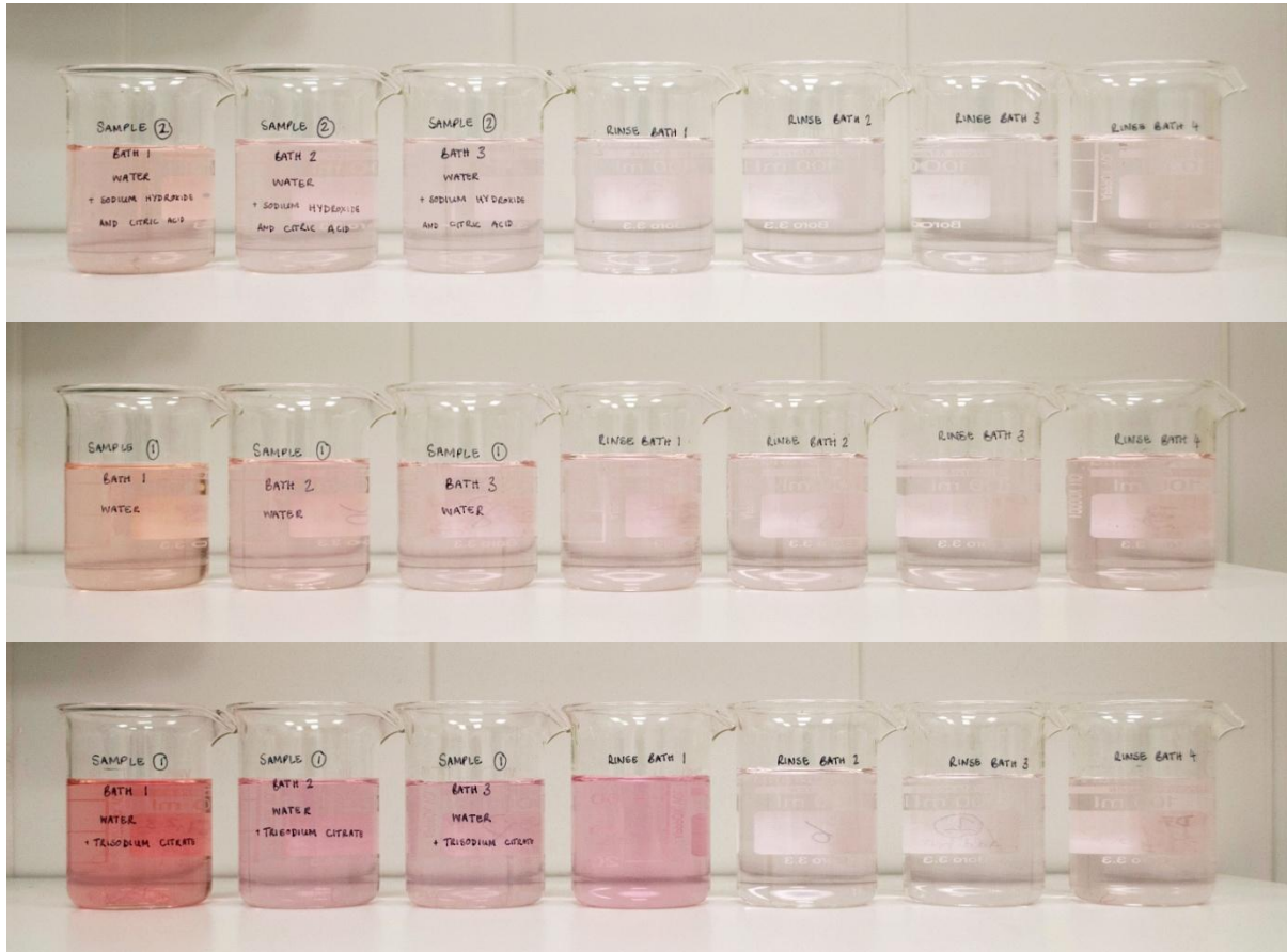
Figure 6.12 Colour difference between wash solution of silk samples WS2 (top), W1 (centre) and WT1 (bottom).
