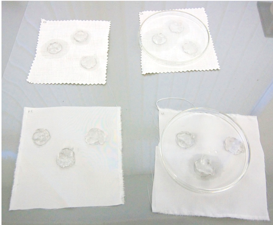
Fig. 8 Monitoring Laponite on cotton and silk. Right side: samples covered with petri dishes
