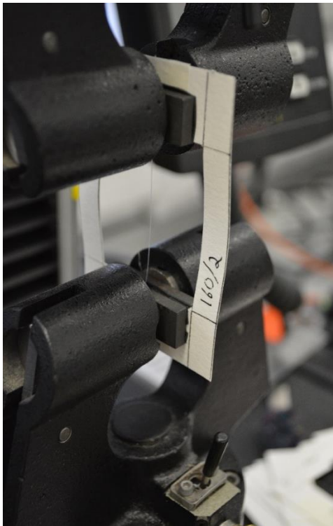
Figure 5.4: Sample clamped in position before testing.
