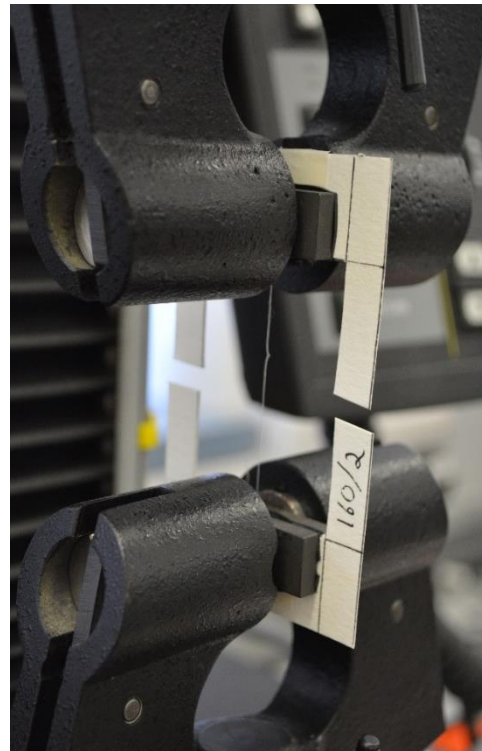
Figure 5.5: Sample clamped in position after testing.
