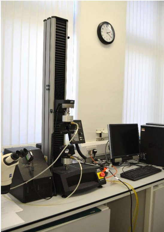
Figure 5.2: Instron 5544 tensile tester and computer with Bluehill software.
