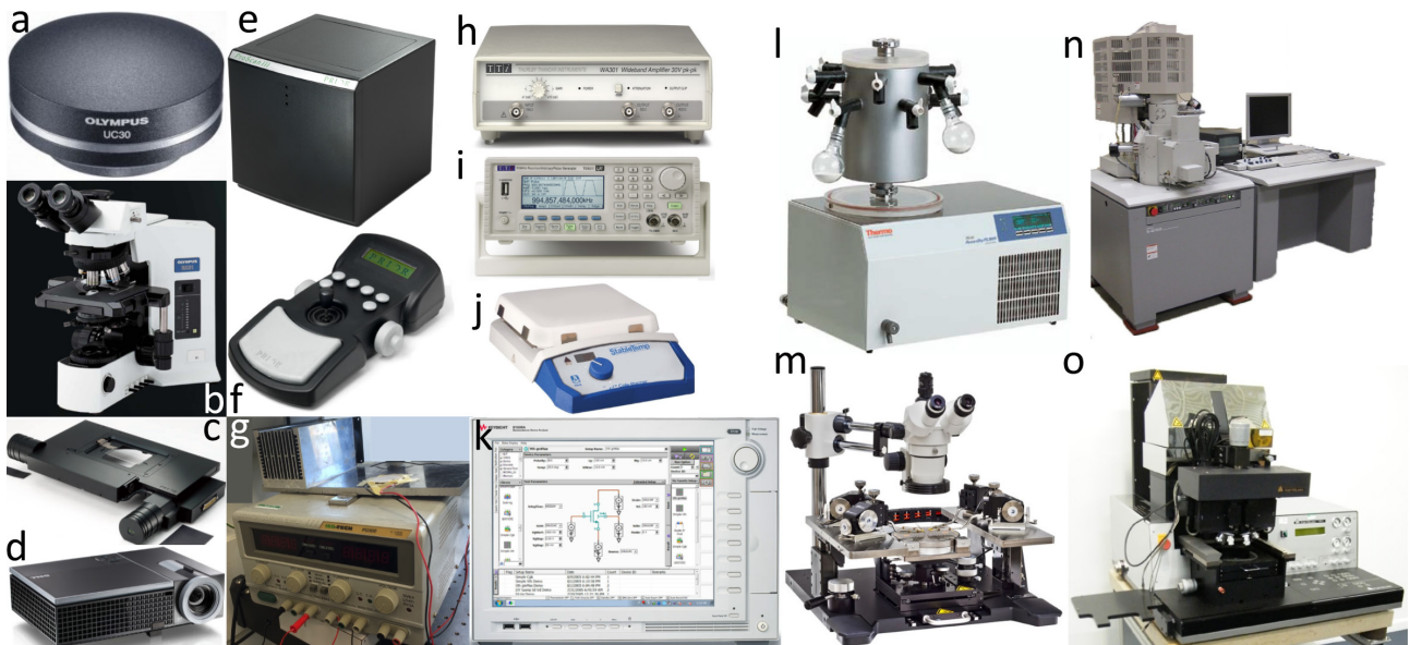
Figure 3.1: (a) Olympus UC30 Microscope Digital Cameras. ref.[70] (b) Olympus BX51. ref.[71] (c) ProScan II H101A stage. ref.[72] (d) Dell 1510X Projector. ref.[73] (e) ProScan III H31 Automation Controller. ref.[74] (f) Proscan III PS3J100 Interactive control Centre. ref.[75] (g) ISO TECH IPS 2303D laboratory DC power supply. ref.[76] (h) TTI TG5011 50MHz function/arbitrary/pulse generator. ref.[77] (i) TTI WA301 Wideband 30V pk-pk amplifier for waveform generation. ref.[78] (j) Cole-Parmer StableTemp Hot Plates. ref.[79] (k) Keysight B1500A Semiconductor Device Analyzer. ref.[80] (l) Thermo Scientific Heraeus PowerDry LL3000 Freeze drying systems. ref.[81] (m) CascadeMicrotech MPS150 Manual Probe System. ref.[82] (n) Hitachi S-4700 SEM. ref.[83] (o) SUSS MicroTec MA6. ref.[84]
