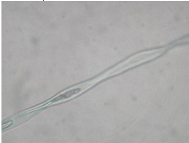
Fig. 27 Photomicrographs: Object 4 Yarn 1: flat, twisted
