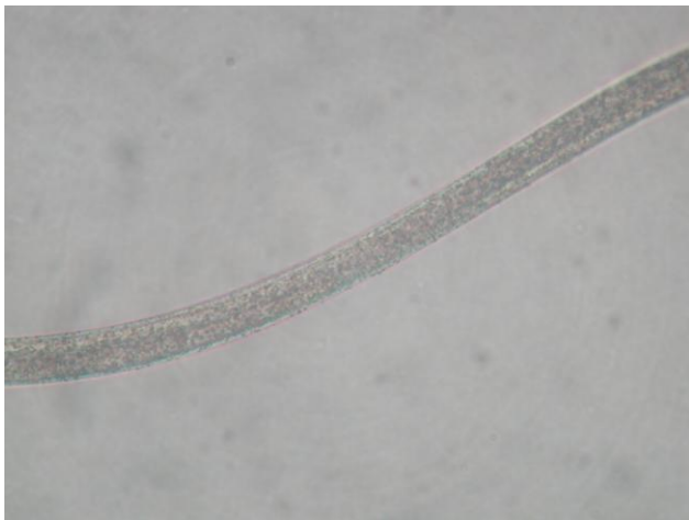
Fig. 35 Photomicrographs: Object 11 Yarn 1: smooth, round, dark specks
