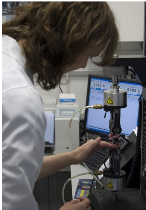
Fig. 46 Mounting Object C test specimen in the Instron device
