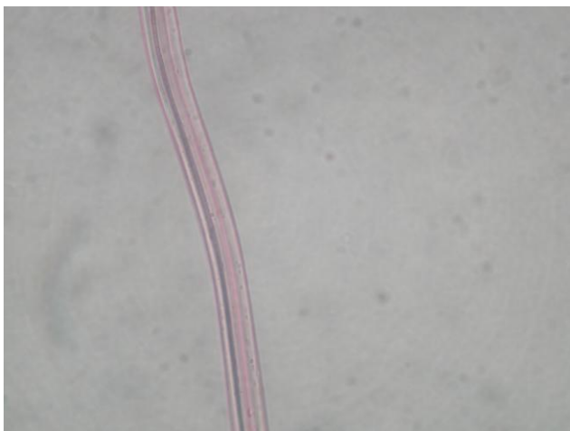
Fig. 30 Photomicrographs: Object 6b Yarn 1: smooth, round, slight striations
