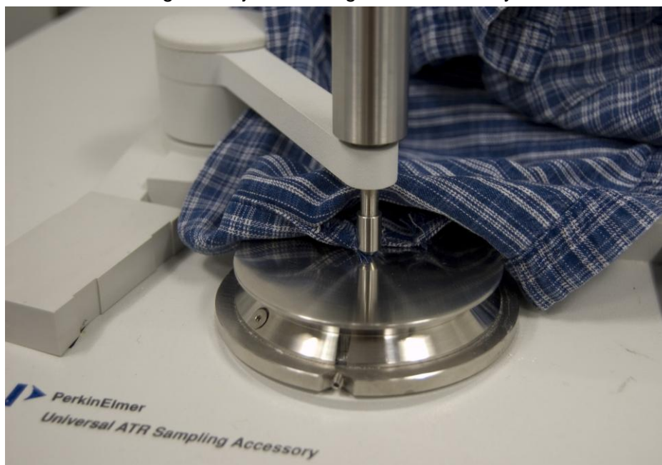
Fig. 38 Object 9 during ATR-FTIR analysis
