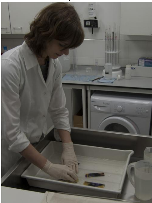
Fig. 44 Conducting wet cleaning treatment on test specimens
