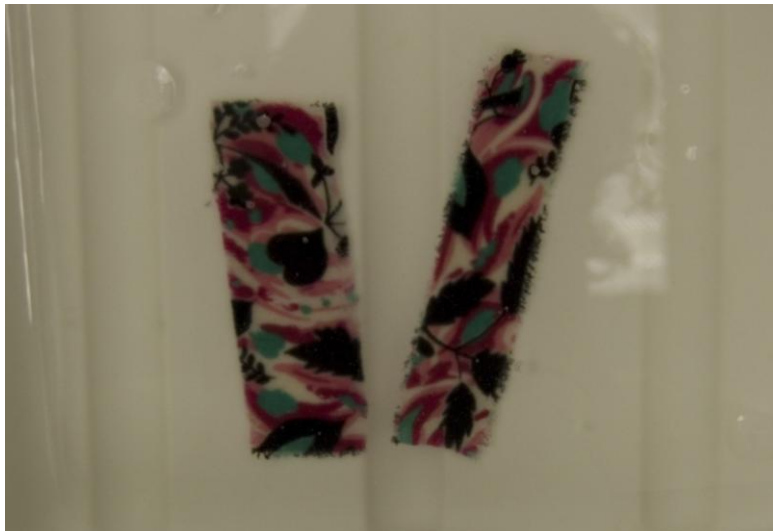
Fig. 60 Visible dimensional change in a warp (left) and weft (right) specimen in the wash bath during Test 2-1-C
