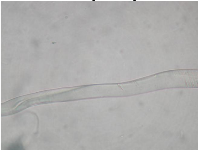
Fig. 24 Photomicrographs: Object 1 Yarn 1: smooth, flat, slight twisting
