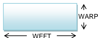
Fig.42 Test specimen cut in the weft direction
