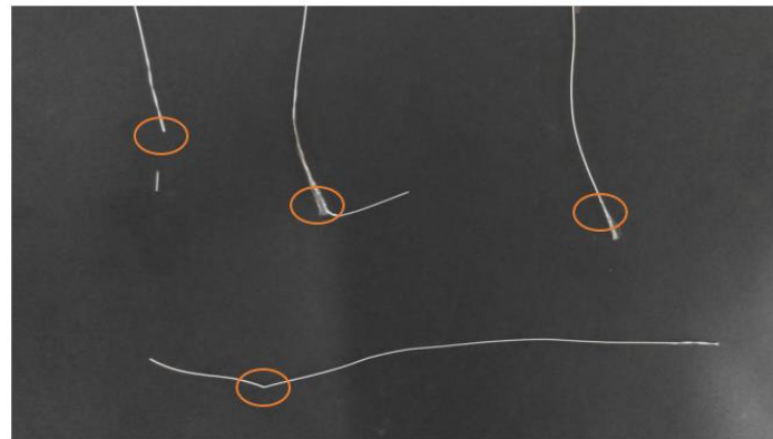
Figure 67: Deformation of coax3 specimens after the UTS test, 1 to 3 (from right to left) above and 4 below the other. Points of failure are spotted in the orange ovoids three.
