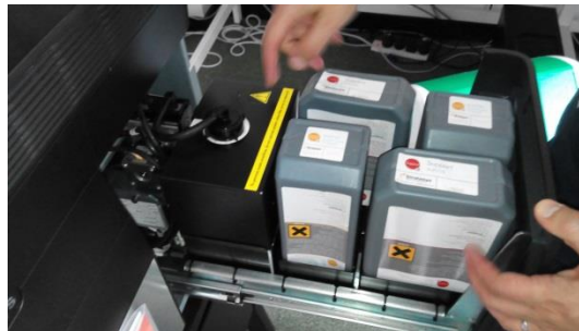
Figure 50: The loading bed for the photopolymer in the Stratasys Objet30 Pro 3D printer
