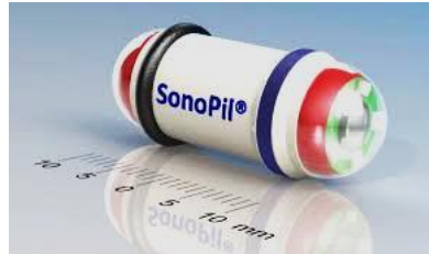
Figure 4: The conception of the Sonopill. The blue ring denotes the position for an ultrasound imaging array and the black ring represents the potential for an autonomous positioning system [25]
