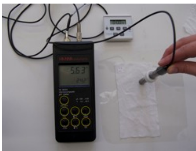
Figure 33: Surface pH Equipment and Method
