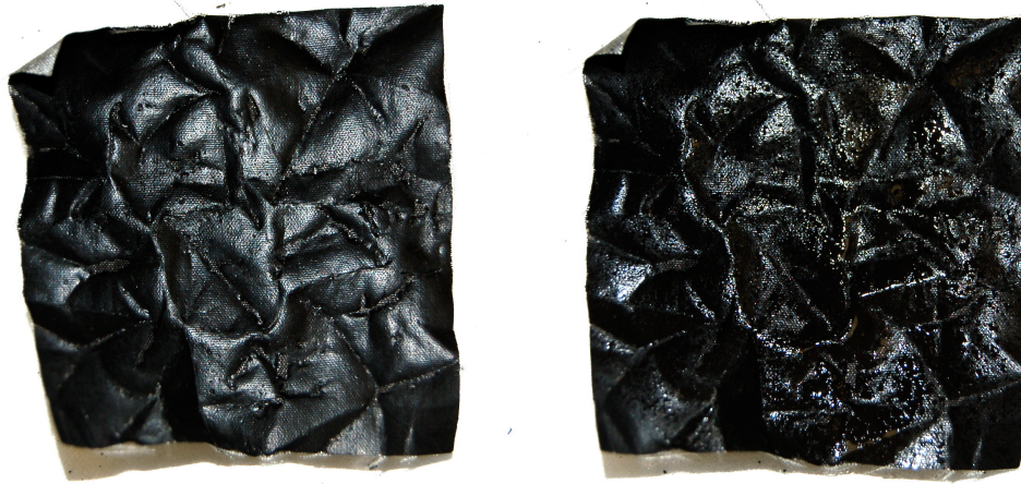
Figure 4.4 – Painted specimen before and after spraying, showing light coat of droplets
