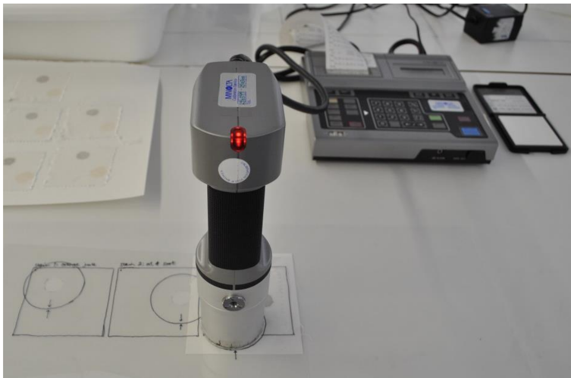
Fig. 6 - Measuring colour readings of a stains test specimen using the Chroma meter
