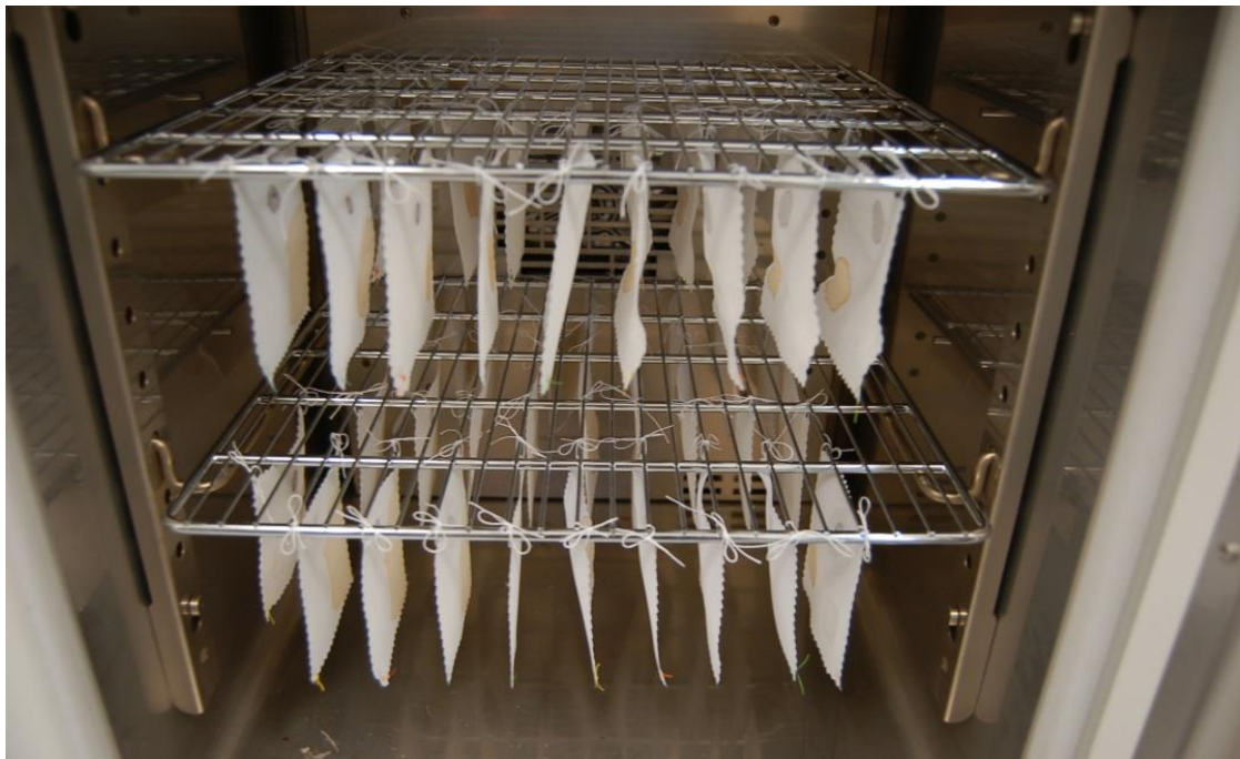
Fig. 3 - Soil removal test specimens in the oven to begin artificial ageing
