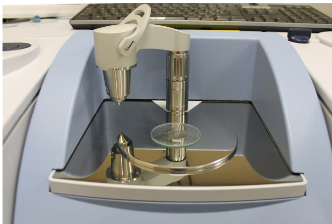
Figure 32 Recording ATR-FTIR spectra of liquid samples
