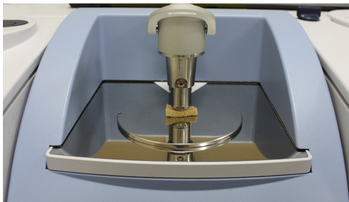
Figure 30 Recording ATR-FTIR spectra of Smoke sponges
