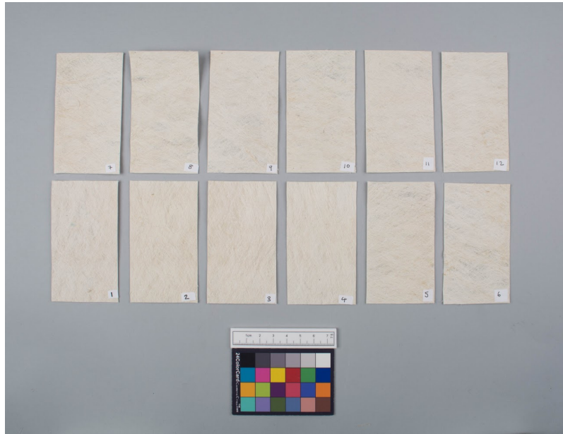
Figure 4: New barkcloth samples prepared for preliminary wash tests.
