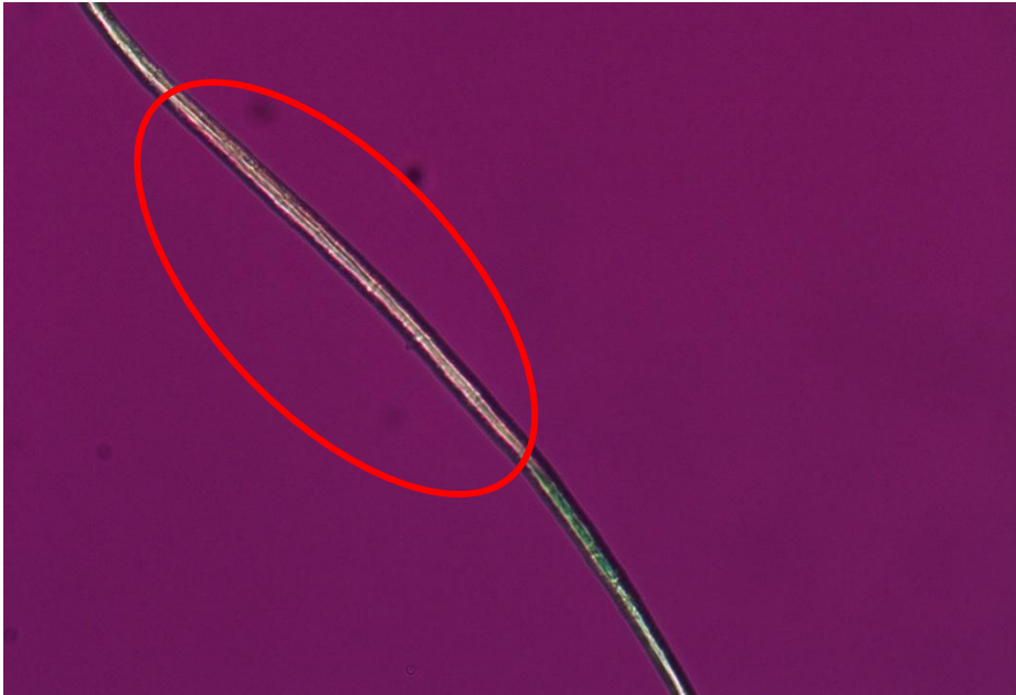
Fig. 20 Stained 15% AA sample AT. Note the fine perpendicular cracks along the fibre.
