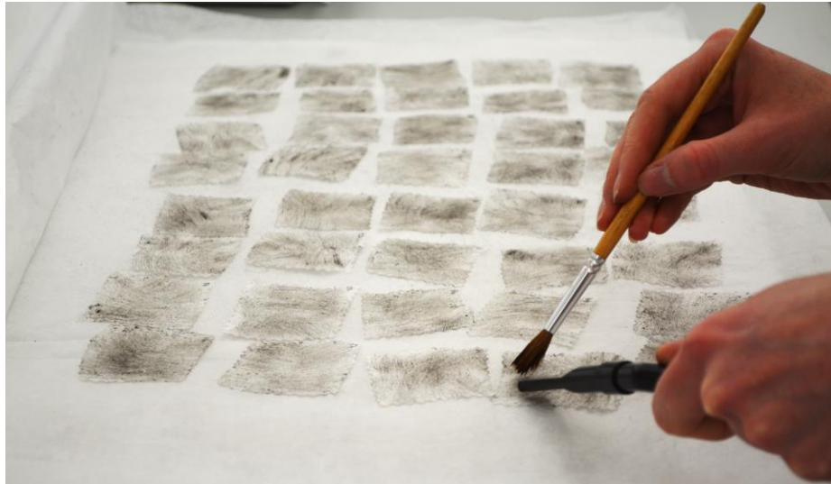
Figure 2: vacuuming the samples to remove any loosely adhered particulate soiling
