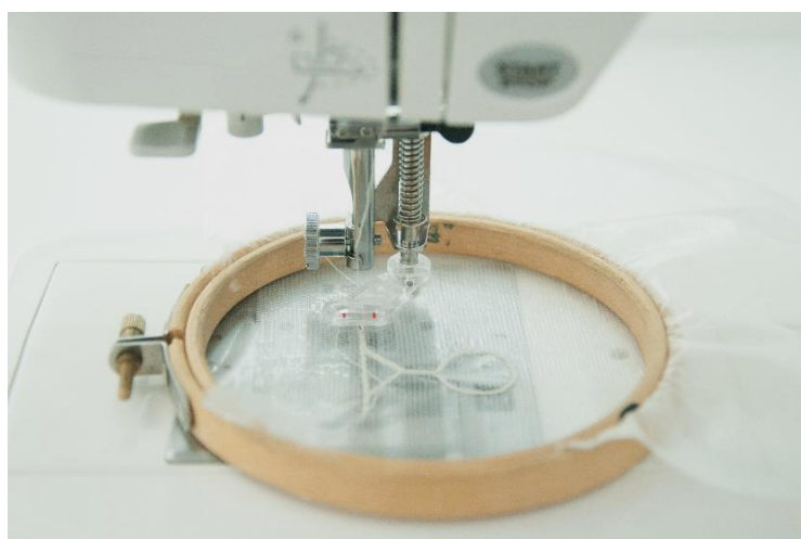
Fig. 8.2.4 Machine sewing through the soluble substrate.
