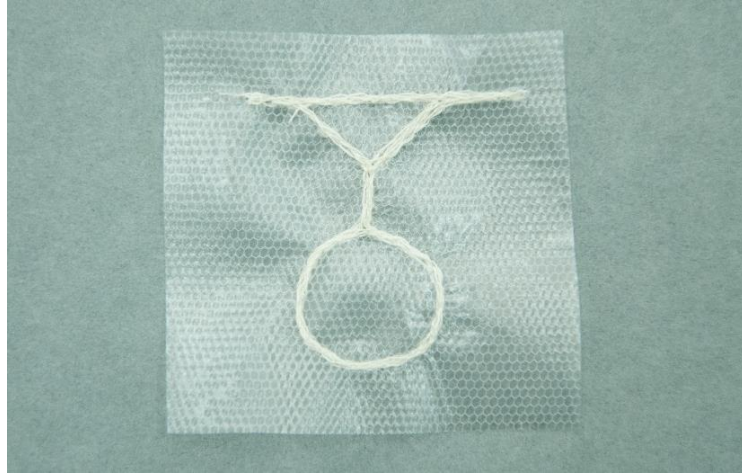
Fig. 8.2.5 Guipure ground before substrate was solubilised.
