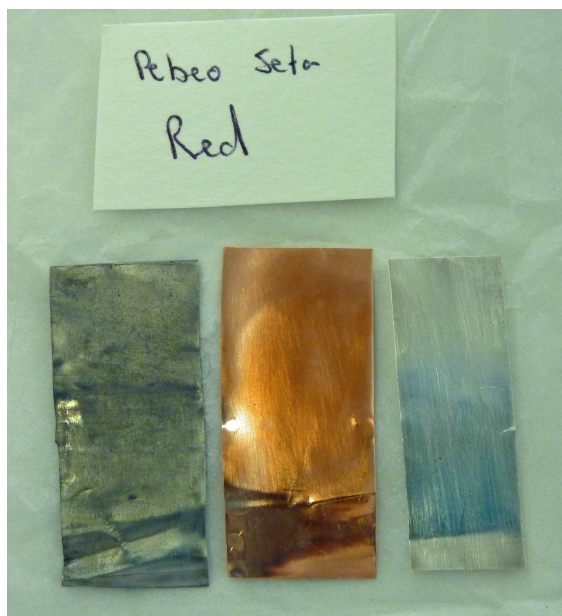
Figure 4: Oddy Test Coupons - Pebeo Setasilk® Red showing some Lead Corrosion
