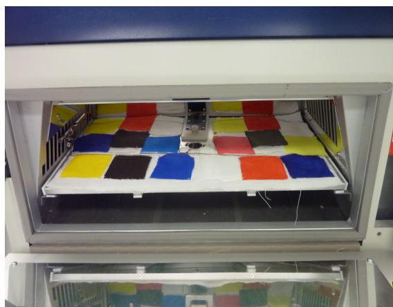
Figure 14: Samples in Q-Sun Light Ageing Testing Chamber.
