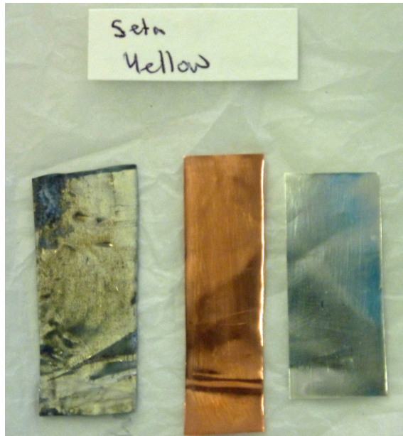
Figure 3: Oddy Test Coupons - Pebeo Setasilk® Yellow, showing Lead Corrosion
