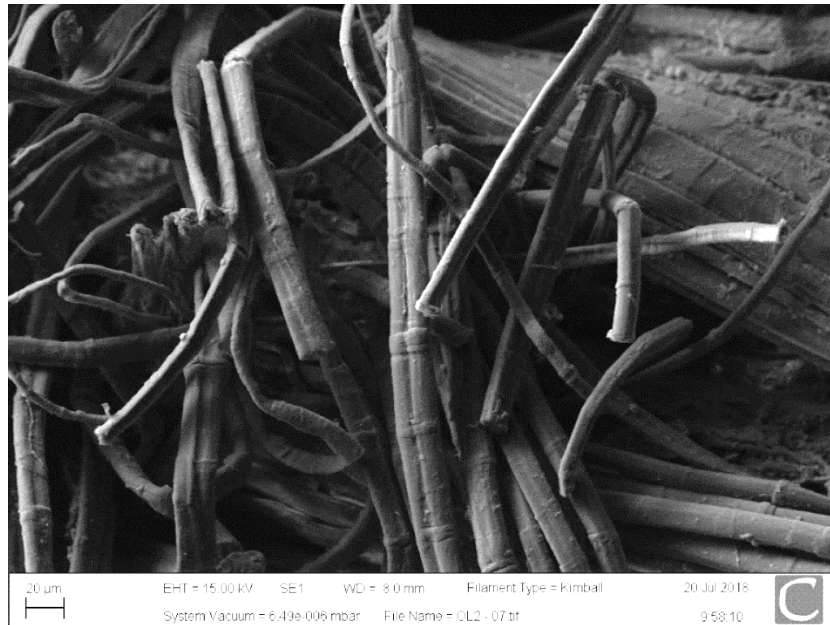
Figure 71 Higher magnification SEM image of historic linen sample OL2 after treatment (no mechanical action).
