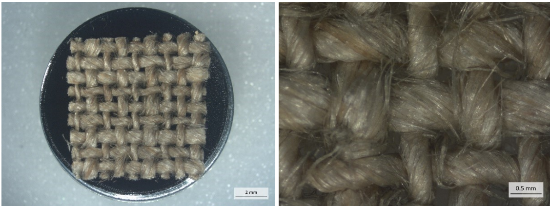
Figure 66 Sample OL5 treated with ultrasound only, appearing slightly darker than samples OL3 or OL4.
