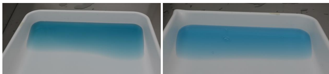
Figures 7.7 and 7.8. Solubilised dye from Sampler 1808 after first (left) and second rinse (right)
