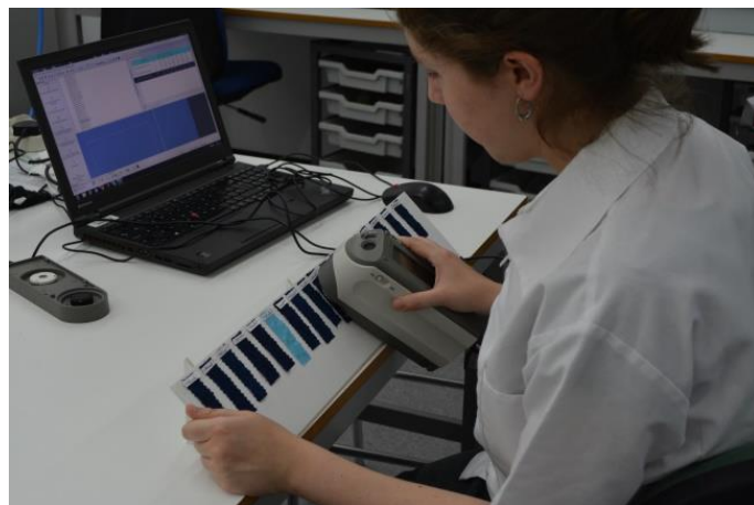
Figure 6.4. Colour measurement of fabric samples with the spectrophotometer
