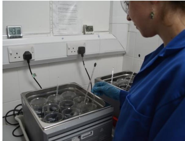
Figure 4.6. Use of two dye-baths with different temperatures
