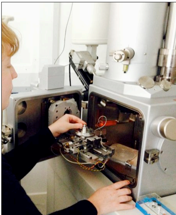
Figure 23: Placing a prepared textile sample in the SEM chamber
