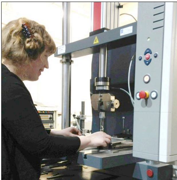
Figure 12: Operating the Tension Compression Machine Zwick/Roell Z2.0
