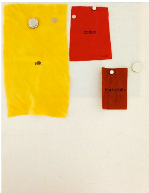
Figure 16: One of two manufactured magnetic display boards – samples were mounted for one month. Environmental conditions were monitored see appendix 7.
