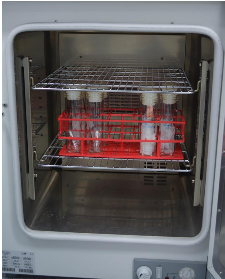
Figure 36: Samples for Oddy test in Heraeus accelerating ageing oven
