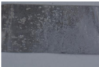
Figure 39: Details of corrosion on lead coupon
