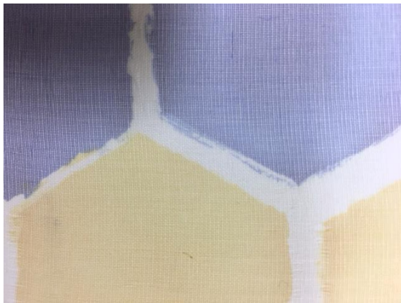
Figure 30: Effects of CDD at edges of fixed dye
