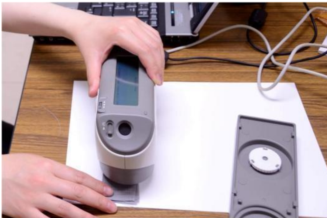
Fig.4-3 Measuring the reflectance value of soiled fabric by spectrophotometer at the KIT.
