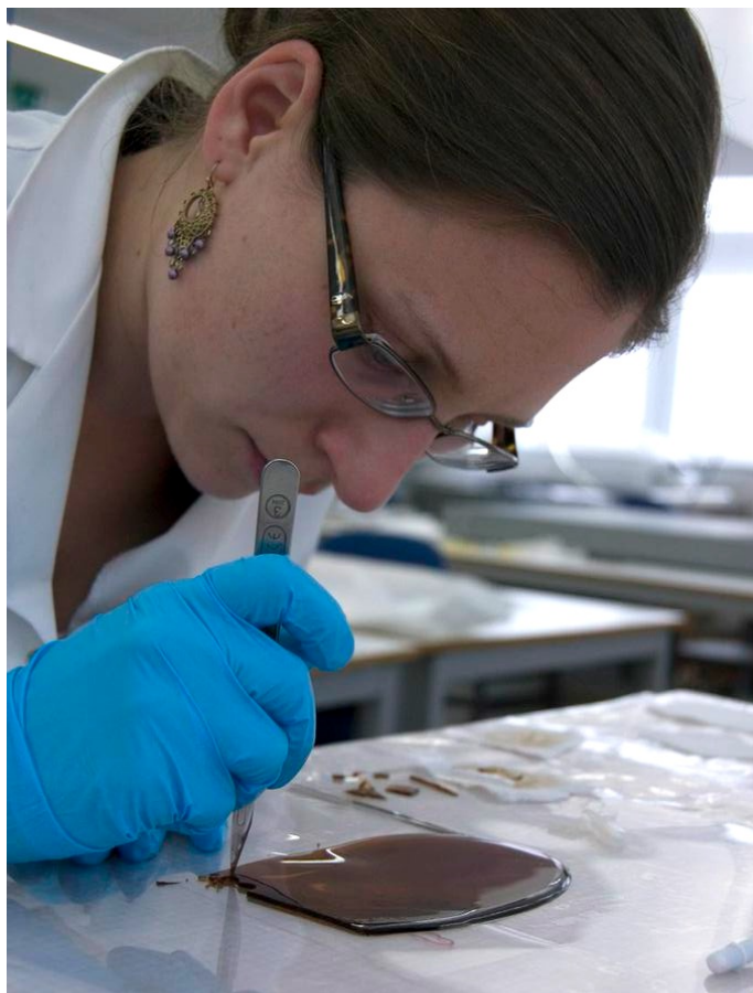
Figure A85: The cast enzyme gel being cut into the shape of the stain. © University of Glasgow
