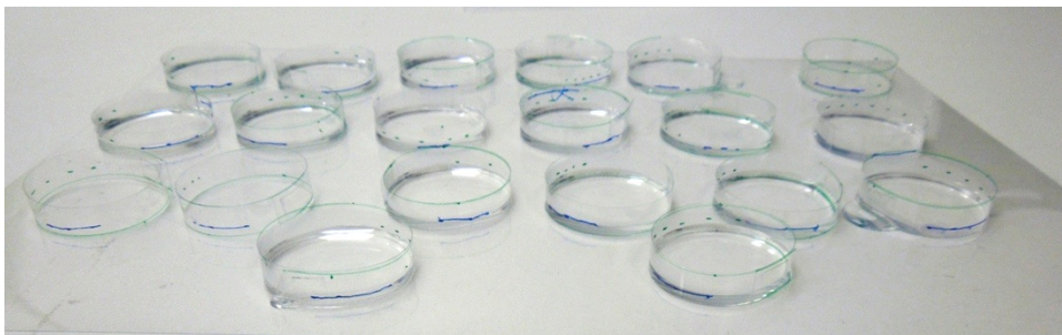
Figure 4: Melinex® rings on Melinex® sheet as used to prepare .3 cm gels.
