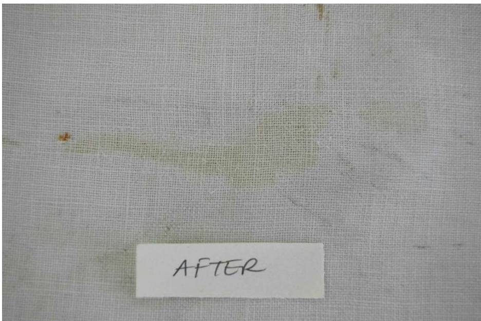
A87: The stain after treatment with the enzyme gel. ©University of Glasgow
