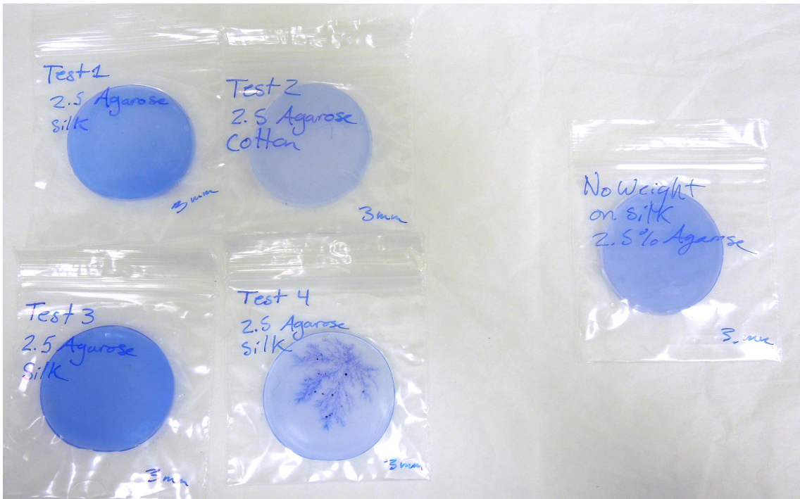
Figure A83: Comparison of weighted and unweighted gels. Left: The 4 tests using .3 cm 2.5% gels applied to silk with weights Right: The .3 cm 2.5% gel applied to silk with no weight
