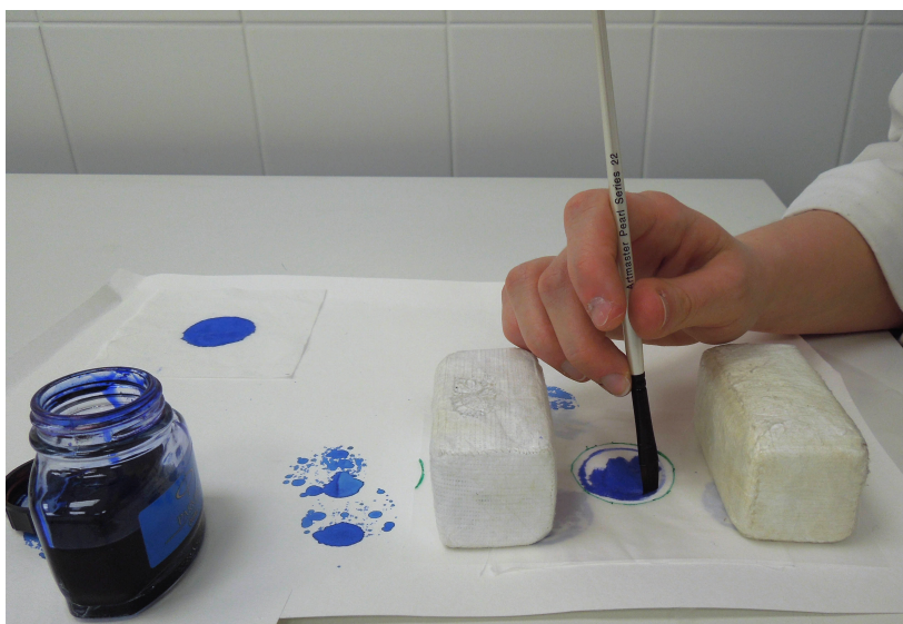
Figure A1: Application of Ink to fabric samples
